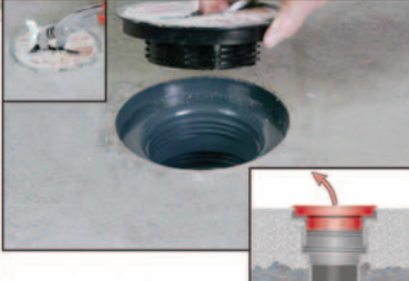
Remove Coring Plug
