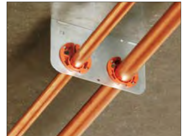
PipeEye Suspension brackets are designed with the same 1-11/32" hole as a standard metal stud punch for use with PipeEye grommets. Secure the brackets directly to ceilings, decks, walls or vent pipes for tight installations where space is limited.
