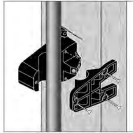
Position pipe. Secure front block to rear block using 1" screws.
