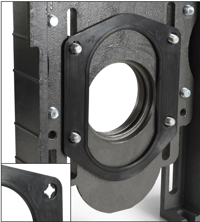
Gasket includes gripping fins to hold fitting screws, keeping both gasket and screws in place during assembly. 'UP' indicator prevents misalignment.
